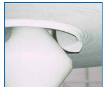
Figure 4: Hooks grab the bottom of the SUPRApak module stack for easy handling.
